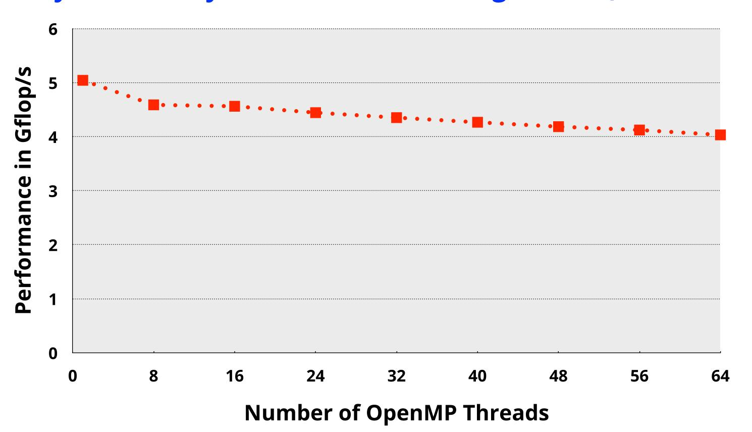
This is a highly parallel algorithm, but adding threads degrades the performance!
