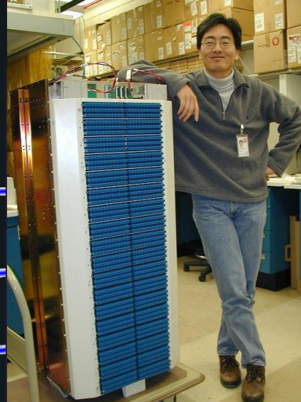
1,100-port photonic switch Jungsang Kim Bell Labs (2002)
